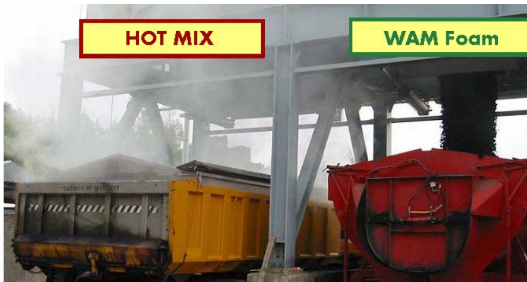
Fig.4 Visual observation of emissions during production of WAM
